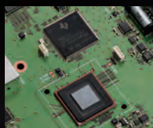
DSP + FPGA Unit (RF Deck)
